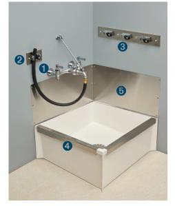
63.600A SERVICE FAUCET – Chrome plated brass service sink faucet, <sup>1</sup>/<sub>2</sub>" pipe eccentric inlets on 8" centers. Vacuum breaker integral stops, chrome plated (H&C) handles, <sup>3</sup>/<sub>4</sub>" hose end spout with pail hook, top reinforcing bar and mounting bracket. Shall meet ANSI Specifications A112.1.1, Section 2.9 and A112.18.1M, CSA Listed. (ANSI)
