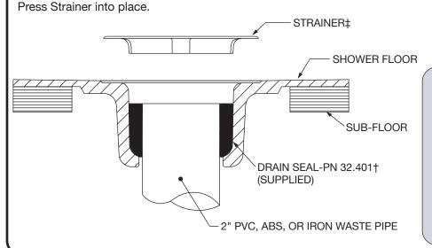
† Optional DRAIN SEALS are available: PN 32.403 - 2" SOIL PIPE/CAST IRON SERVICE WT. (NO HUB)
