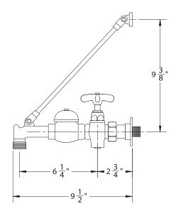
**General:** Chrome plated brass service sink faucet, ½" pipe eccentric inlets on 8" centers. Vacuum breaker integral stops, chrome plated (H&C) handles, ¾" hose end spout with pail hook, top reinforcing bar and mounting bracket. Shall meet ANSI Specifications A112.1.1, Section 2.9 and A112.18.1M, CSA Listed. Install as shown on plans and in accordance with local codes.
